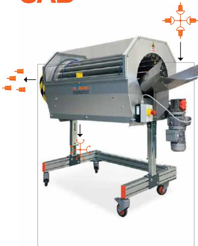
Drum sprue separator, made in electro-welded tubular structure to separate sprues from moulded parts of different thickness, placed near the machine under the loading conveyor. The drum unit is available with rotating rollers (manual adjusting of the distance between rollers) or with punched drum (holes diameter according to our technical department).
