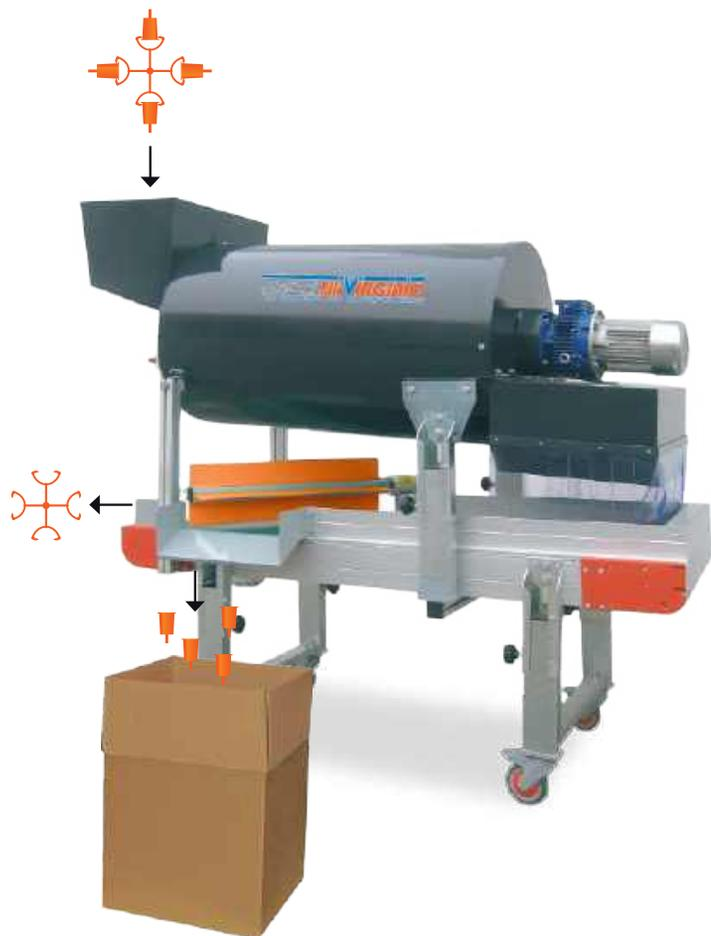
Sprue separator made of metal sheet and aluminium, to divide the moulded parts from the sprues, with adjustable speed by handwheel. Equipped with conveyor belt with paddle separator or roller separator to sort the divided parts.
