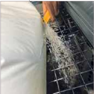
Detail: grid for bag support Particolare: griglia poggia sacco
