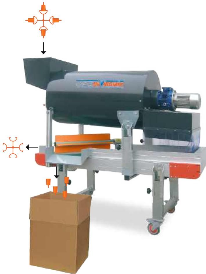
Sprue separator made of metal sheet and aluminium, to divide the moulded parts from the sprues, with adjustable speed by handwheel. Equipped with conveyor belt with paddle separator or roller separator to sort the divided parts.
