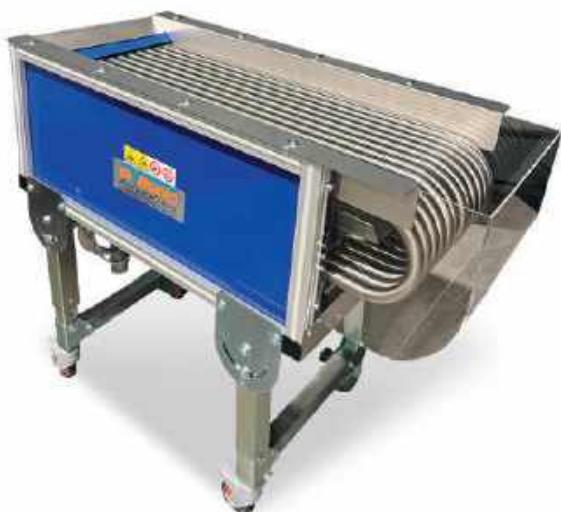
Vibrant sprue separator, made in stainless steel structure to separate the sprues from moulded parts of different thickness, placed near the machine under the loading conveyor. The separator unit is equipped with pipes which by the vibration allow the separation of the parts.
