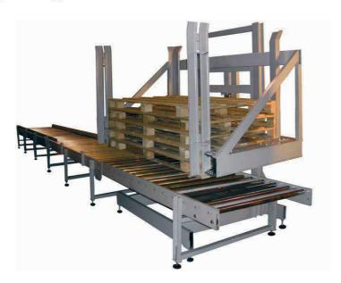
conveyor belt with automatic palletizer system
