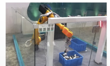
► Three-dimensional round tube to realize random picking
