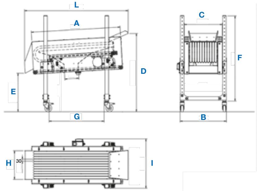
Vibrant sprue separator, made in stainless steel structure to separate the sprues from moulded parts of different thickness, placed near the machine under the loading conveyor. The separator unit is equipped with pipes which by the vibration allow the separation of the parts.
