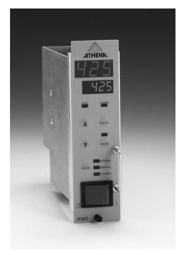
The Athena Series RMB is a microprocessor-based, single-zone temperature controller specifically designed for runnerless molding applications. It features an easy-to-use operator keypad, two LED displays, and three discrete indicators for heat-current, alarm and manual mode.
